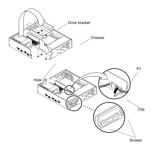
FIGURE 2-13 Positioning the Drive Bracket in the Chassis
