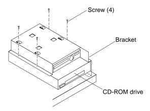
FIGURE 2-11 Positioning the CD-ROM Drive
