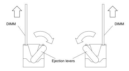
FIGURE 2-7 DIMM Ejection Levers
