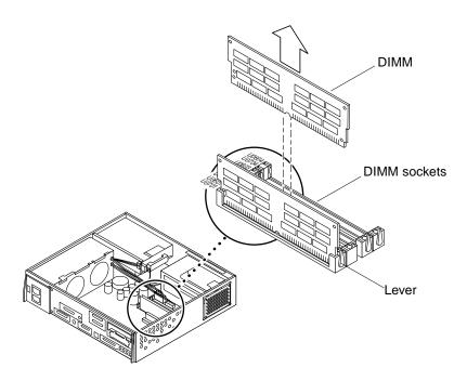
FIGURE 2-8 Removing a DIMM
