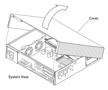
FIGURE 2-3 Removing the Cover
