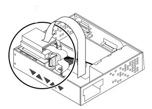
FIGURE 2-12 Replacing the Drive Bracket in the Disk Drive Bay
