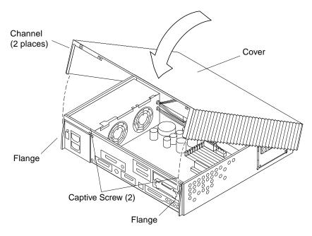
FIGURE 2-14 Replacing the Cover
