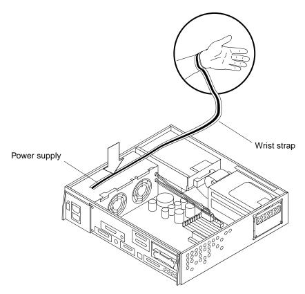
FIGURE 2-4 Attaching the Antistatic Wrist Strap
