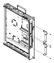
FIGURE 10 PCI Front Bracket Installation
