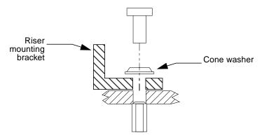
FIGURE 15 Cone Washer and Standoff
