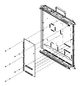
FIGURE 3 SBus I/O Module Removal
