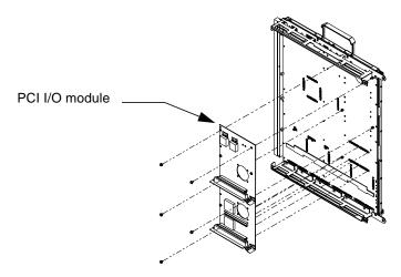
FIGURE 13 PCI I/O Module Installation
