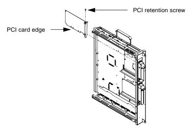
FIGURE 17 PCI Card Installation
