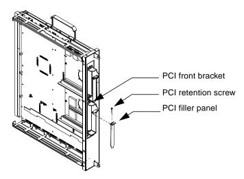
FIGURE 11 PCI Filler Panel Installation
