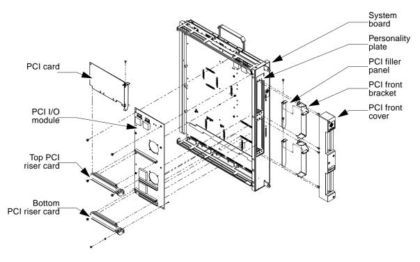
FIGURE 9 PCI Components
