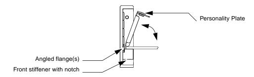
FIGURE 5 Personality Plate Removal (Top View)
