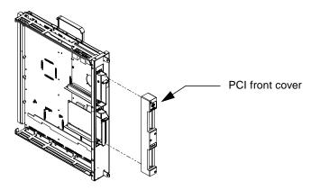
FIGURE 18 PCI Front Cover Installation
