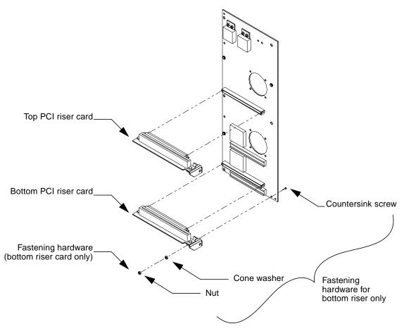
FIGURE 12 PCI Riser Card Components
