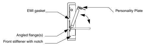
FIGURE 7 Personality Plate Installation (Top View)
