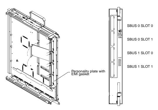
FIGURE 2 SBus Card Removal
