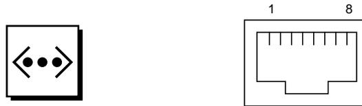
FIGURE 4-4 RJ45 TPE Socket
