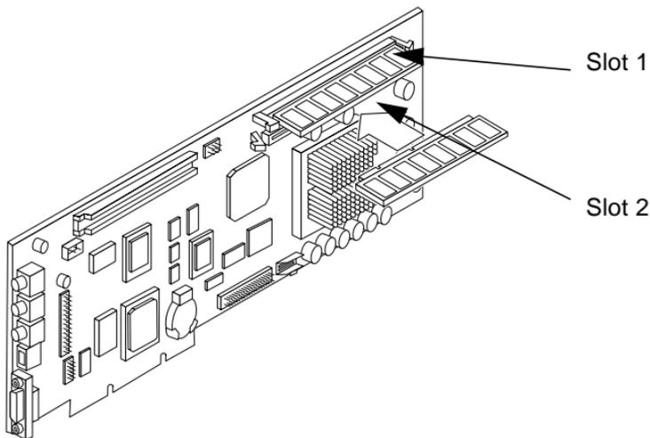
**FIGURE 1** Locating DIMM Slots on the SunPCi Card
