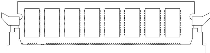
**FIGURE 2** Properly Installed DIMM
