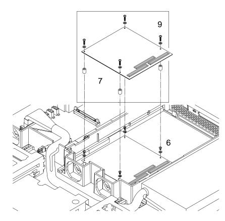
There is one memory board in the shipped system. You can upgrade it and install an additional memory board.
