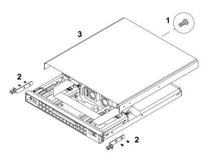
1 Remove the cover screw using a Phillips No. 2 screwdriver. 2 Remove the rack brackets, if fitted. 3 Slide the cover to rear and lift. 4 Reverse the procedure to replace the cover. See panel 9 for more information about disassembling the system when required to install options.
