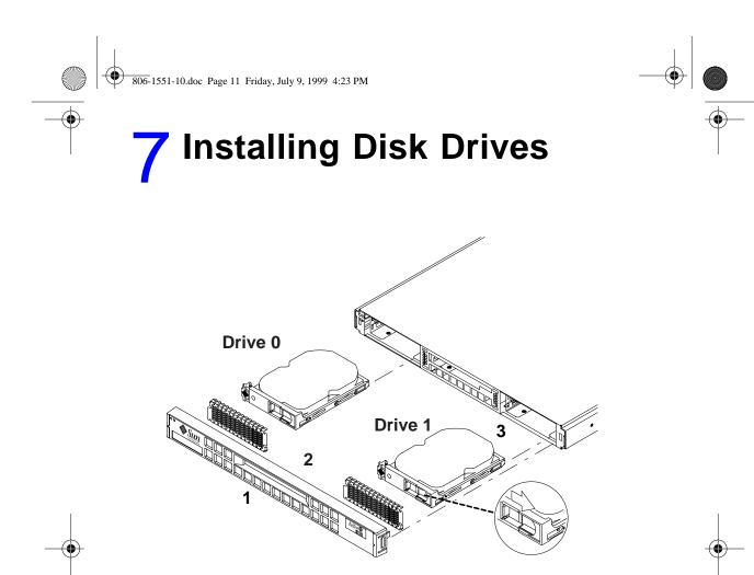
1 Remove the front bezel by pressing the latch at either end. 2 Lever the grilles out. 3 Slide the disk drive(s) in to the front of the system. 4 Replace the grilles and front bezel.
