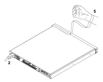
1 Shut down Solaris<sup>™</sup> from the console. 2 Turn the power supply switch off. 3 Disconnect the AC power cord. 4 Disconnect any other cables. 5 Remove the system from the rack and place at an ESD station. 5 Attach the wrist strap to the attachment point on the station.
