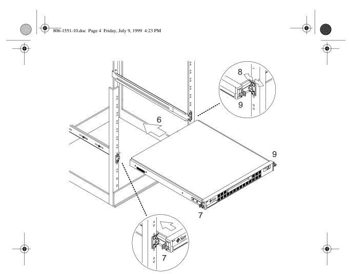
6 Slide the unit into the rack. 7 Fasten the screws on the left side of the unit. 8 Adjust the bracket on the right side of the unit. 9 Fasten the screws on the right side of the unit. It may be necessary to readjust the brackets fixings in order to align the system as required.
