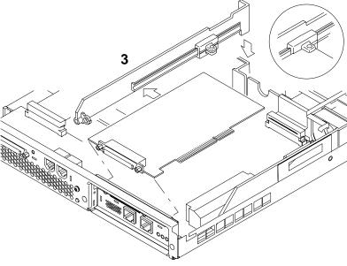
See panel 9 for an illustration of all removable parts. 1 Remove the system from the rack (see panel 4). 2 Remove the cover (see panel 4). 3 Push the slide in the mid-baffle away from the edge of the PCI card and lift out the baffle. 4 Remove the blanking panel or previous PCI card. 5 Slide the PCI card into place. 6 Insert the mid-baffle. 7 Push the slide in the baffle forward to hold the PCI card in place. 8 Replace the other components in the reverse order to that in which you removed them.
