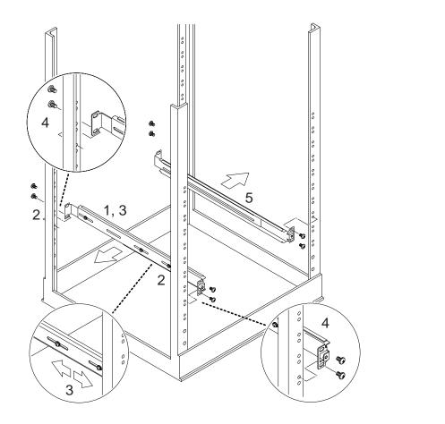
1 Slacken the M4 nuts on the left bracket. 2 Adjust the bracket to fit the rack. The ends of the bracket must be outside the rack. 3 Move the brackets so that the studs are in suitable slots and tighten the nuts. 4 Fasten the screws on both ends of the bracket. 5 Repeat for the right bracket.
