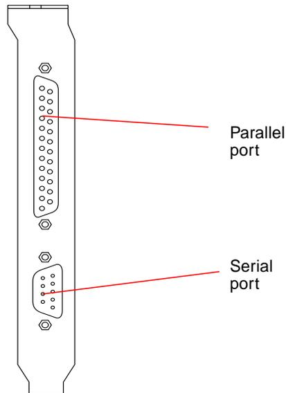
**FIGURE 10-2** SunPCi II Card Add-On Backplate Connectors
