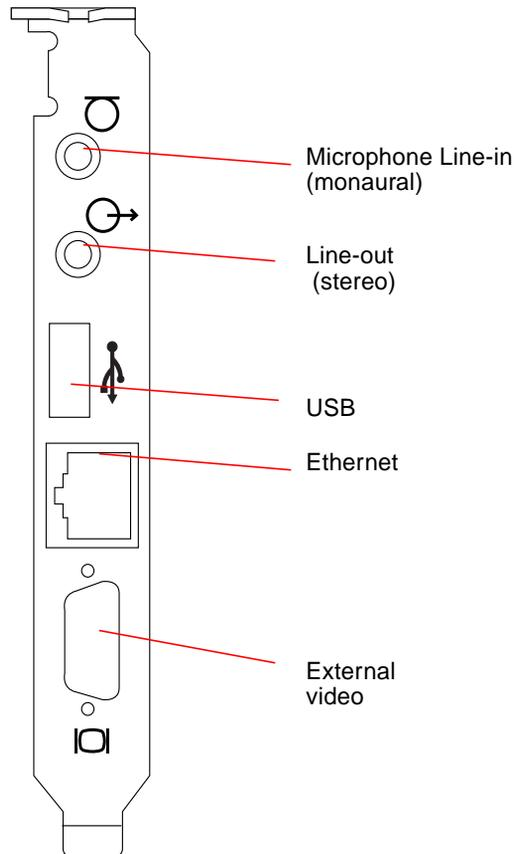
**FIGURE 10-1** SunPCi II Card Backplate Connectors
