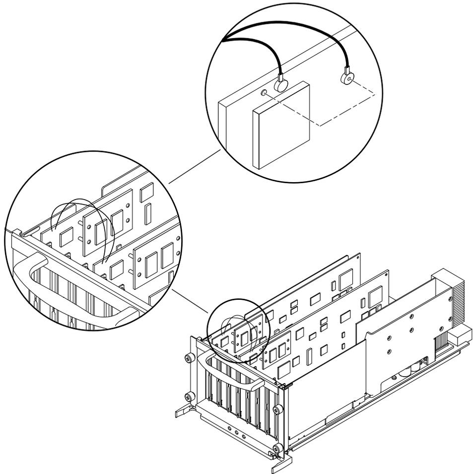
**FIGURE 4-3** Detail of the SRP Clock Cables Connecting Two Sun OC48 Packet Over Sonet Adapters
