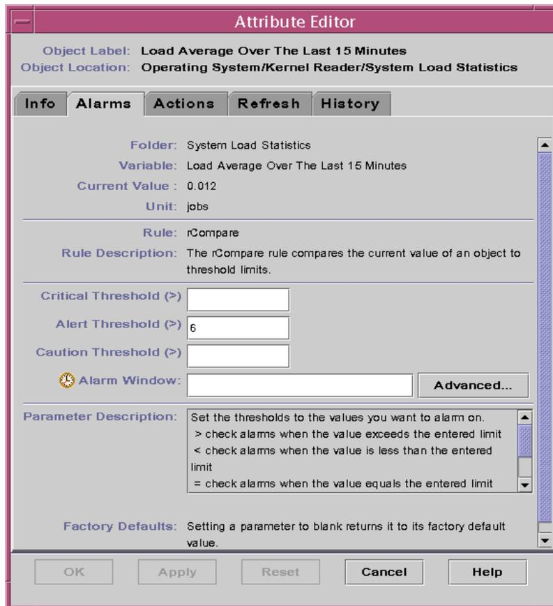
FIGURE 4-11 Alarm Threshold Information
