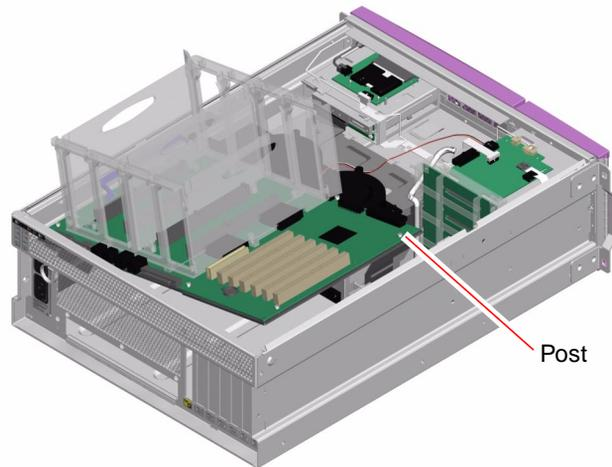
2. Tighten the ten Phillips No. 2 captive screws to secure the motherboard to the chassis.
