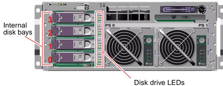
Listed from top to bottom, the disk drive LEDs operate as described in the following table.
