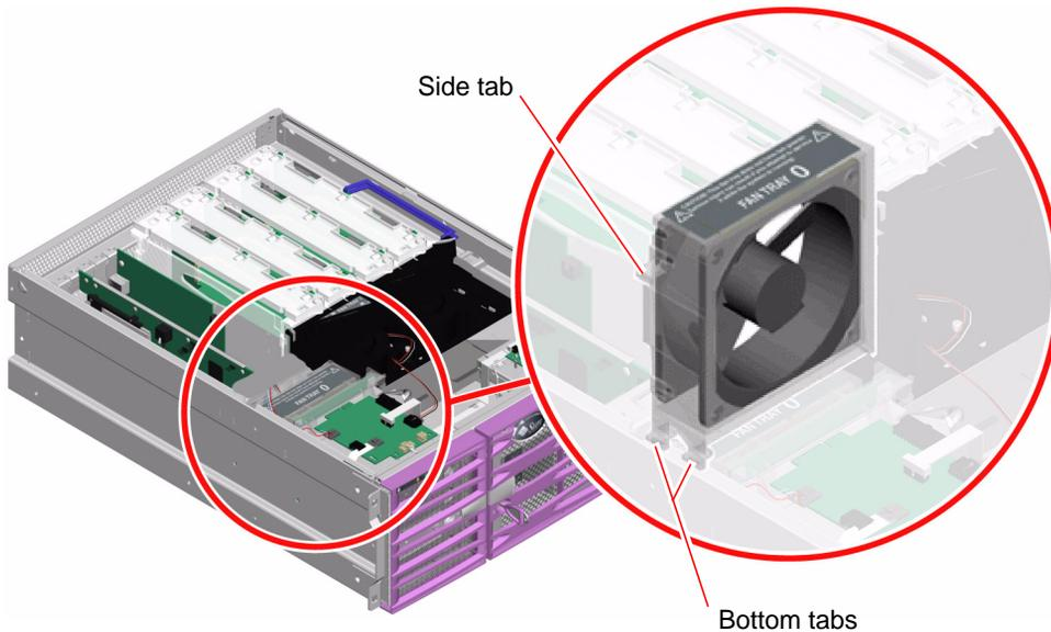
2. Insert the PCI fan tray into the system until it is firmly seated.
