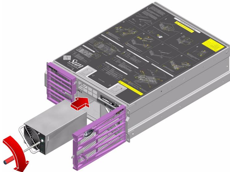
**4. Push firmly on the front of the power supply to engage the power supply connectors with the motherboard connectors.**
