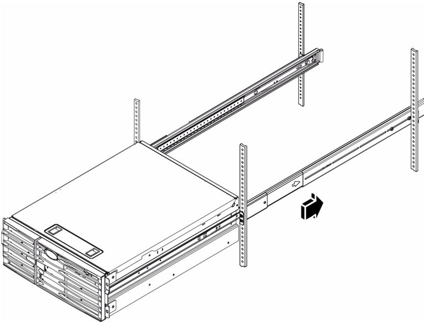
**3. Tighten the four captive screws that secure the system to the left and right vertical rails at the front of the cabinet.**
