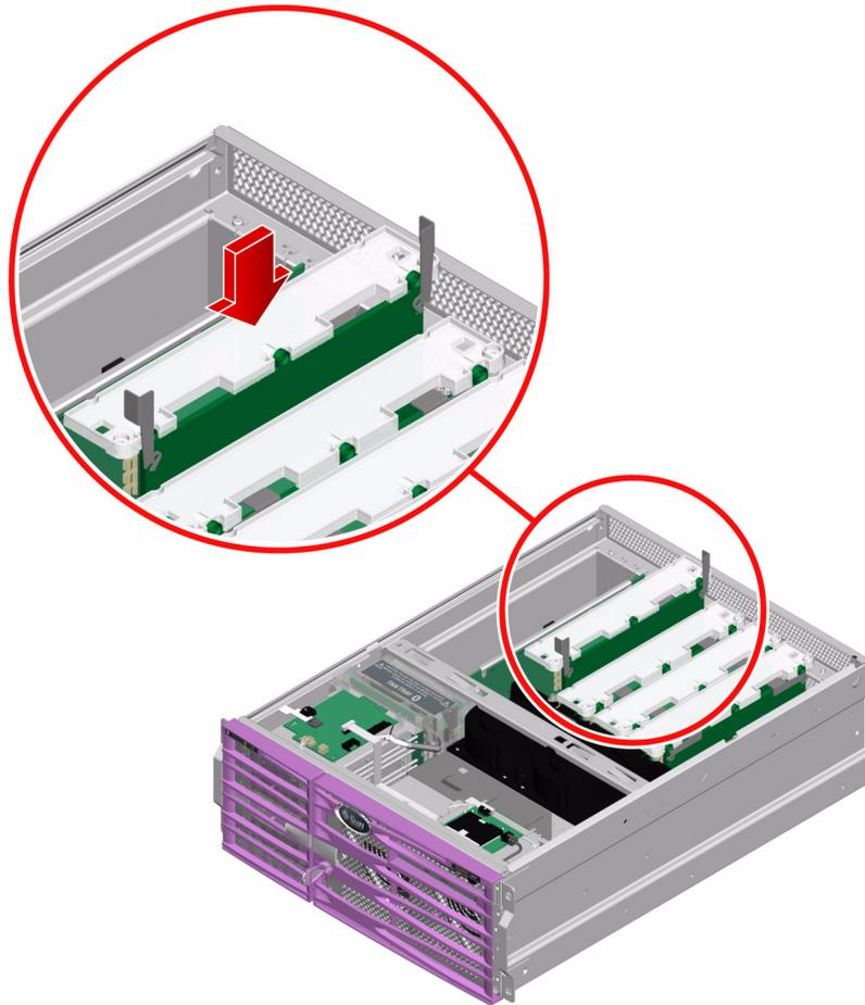
**5. Push down on both ejector levers, simultaneously, until the levers are completely pressed into their slots.**
