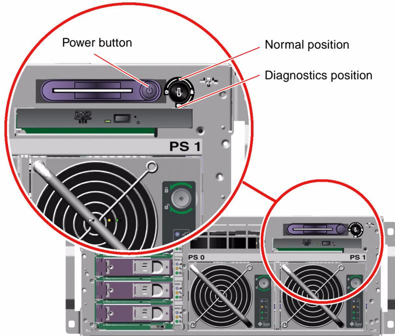
**6. Press the Power button that is to the left of the system control keyswitch to power on the system.**
