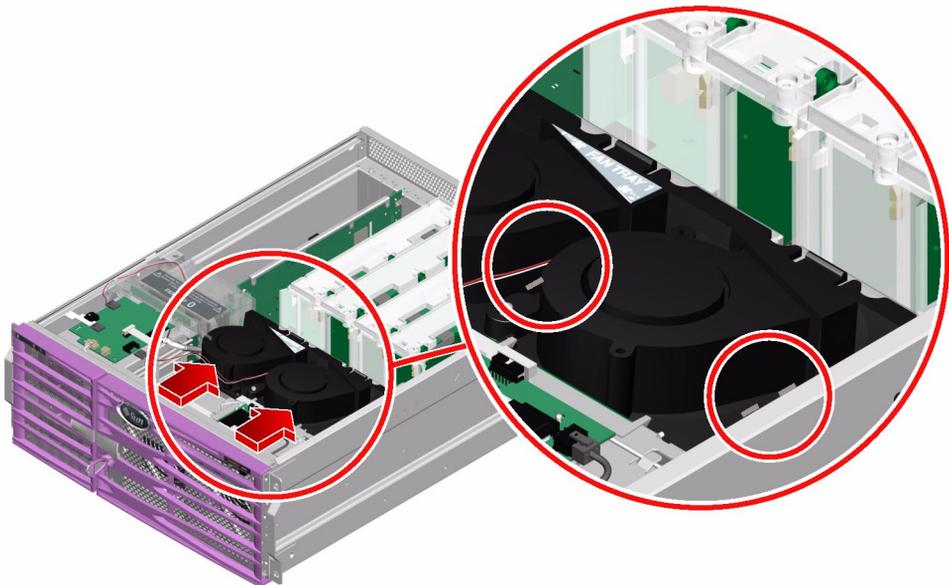
3. **Tighten the Phillips No. 2 captive screw that secures the CPU fan tray to the chassis.**
