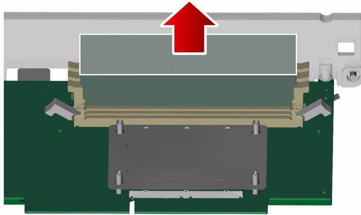
4. Place the memory module on an antistatic mat.
