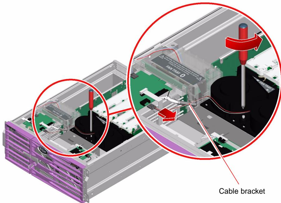
5. Remove the cable assembly from the cable bracket on the side of the SCSI backplane.
