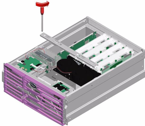
4. Disconnect the PCI fan tray cable at P7 on the connector board.
