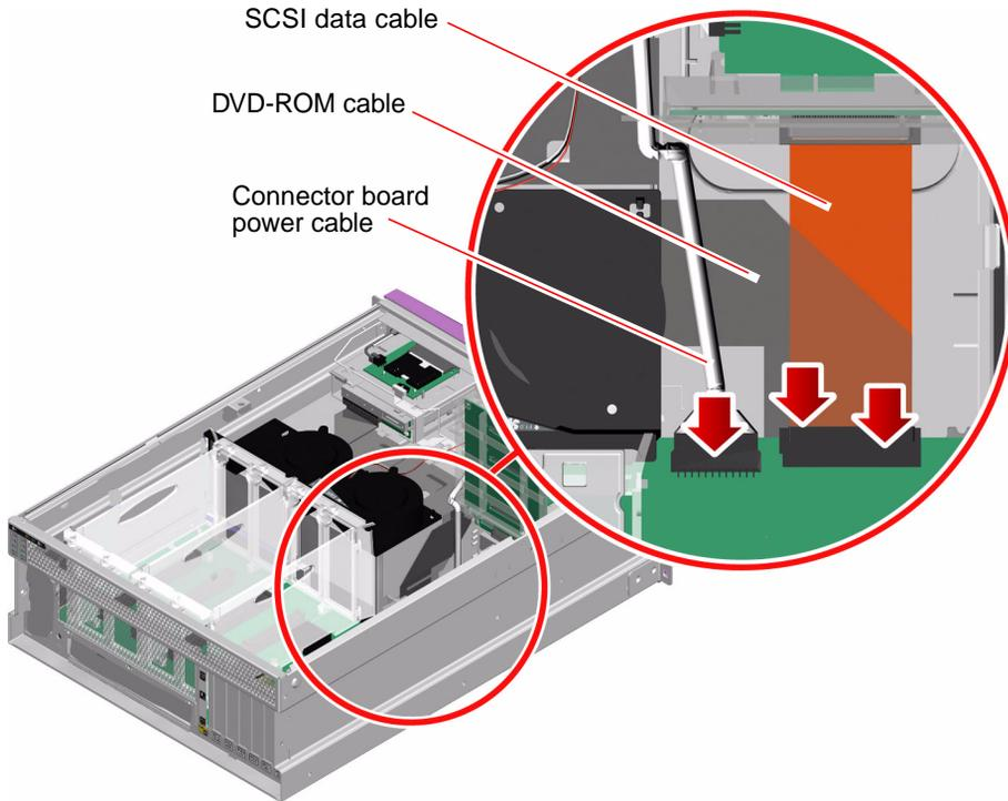
5. Connect the P5 connector board power cable end at P5 on the motherboard.
