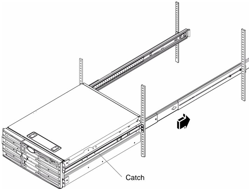
5. Slide the system evenly into the cabinet until the system stops moving.
