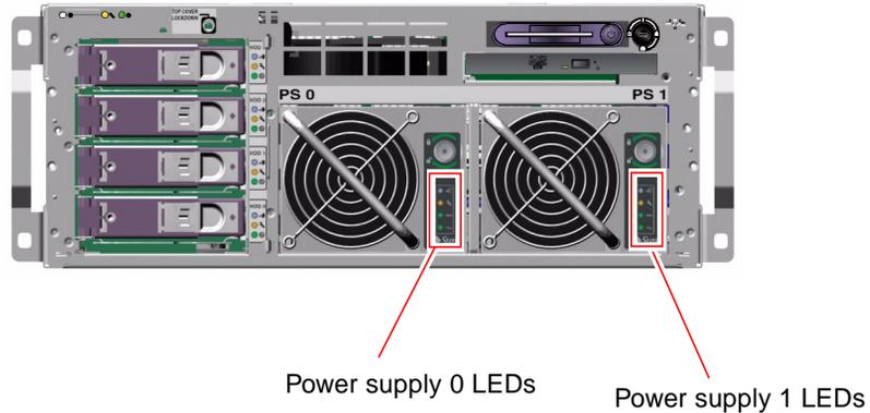
Each power supply LED has a corresponding LED on the back panel.
