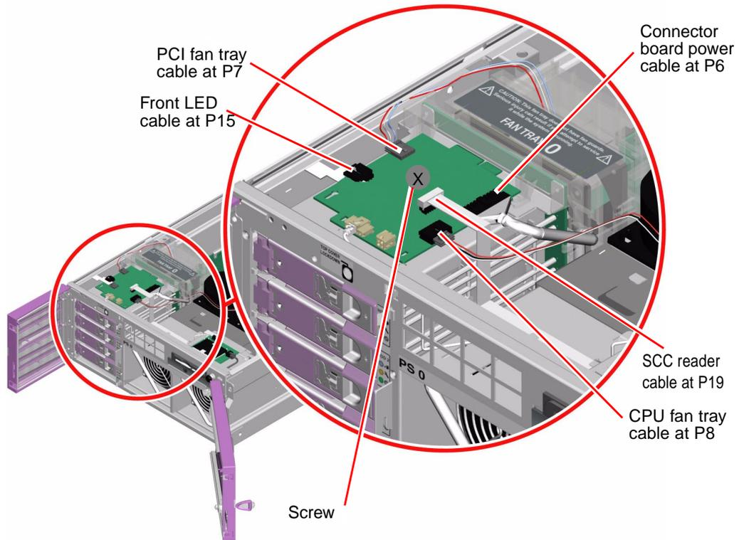
**3. Loosen the Phillips No. 2 captive screw securing the connector board to the chassis.**
