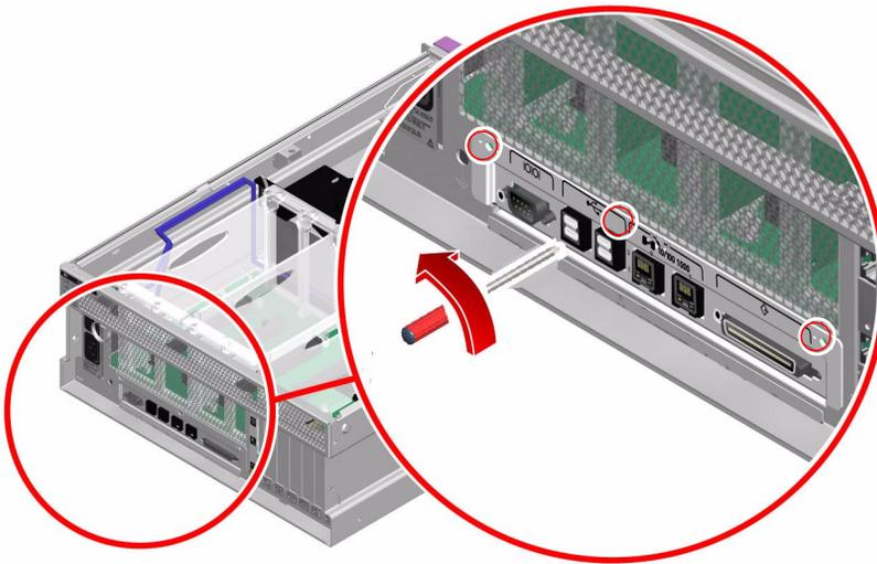
**5. Disconnect the P5 connector board power cable end at P5 on the motherboard.**
