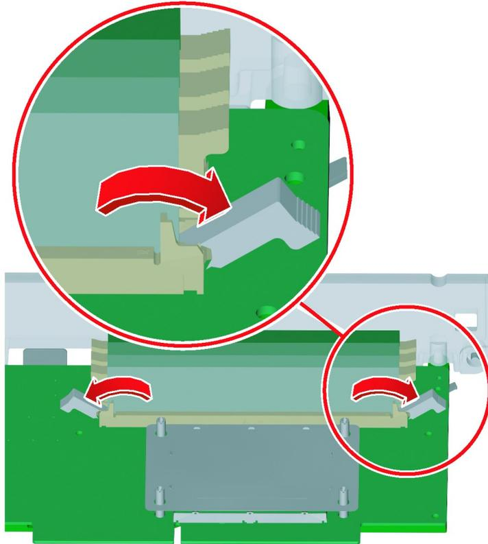
3. Grasp the top corners of the memory module and pull it up and out of its socket.
