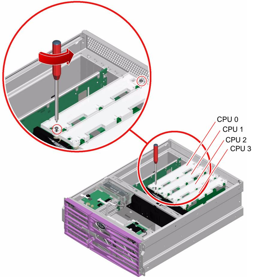
3. Rotate the CPU/memory module ejector levers upward so that the CPU/memory module connectors disengage from the CPU cage.
