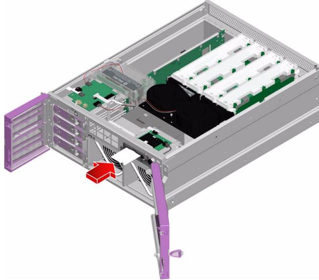
2. **Insert the security post into its position in front of the SCC.**
