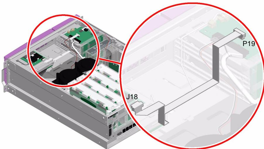
3. Tuck the cable under the two metal tabs located on the chassis above power supply 0.
