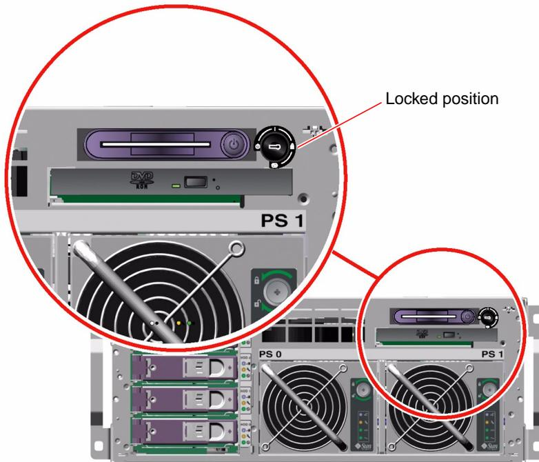
**8. Remove the system key from the system control keyswitch, close and lock the system doors, and keep the key in a secure place.**
