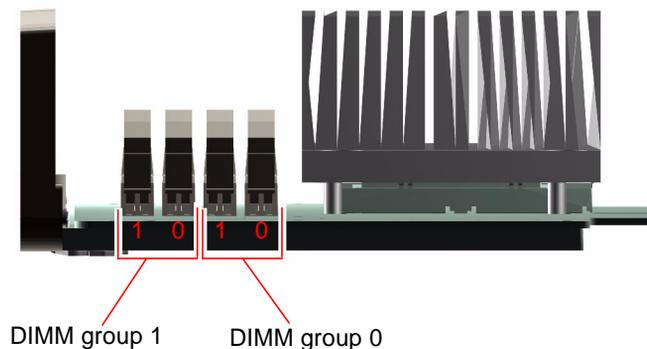
You must physically remove a CPU/memory module from the system before you can install or remove DIMMs. The DIMMs must be added in pairs within the same DIMM group, and each pair used must have two identical DIMMs installed—that is, both DIMMs in each group must be from the same manufacturing vendor and must have the same capacity (for example, two 512-Mbyte DIMMs or two 1-Gbyte DIMMs).
