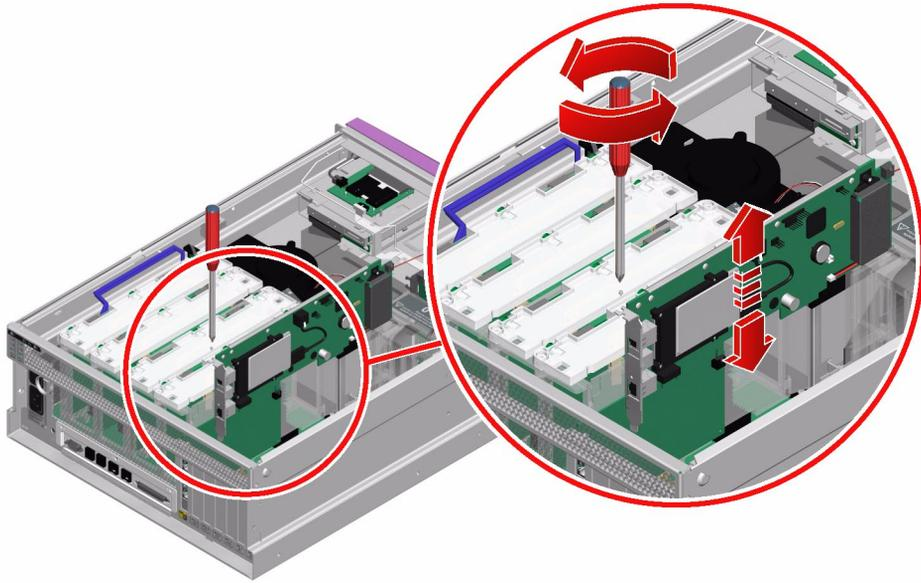
4. Pull the PCI card from its slot.
