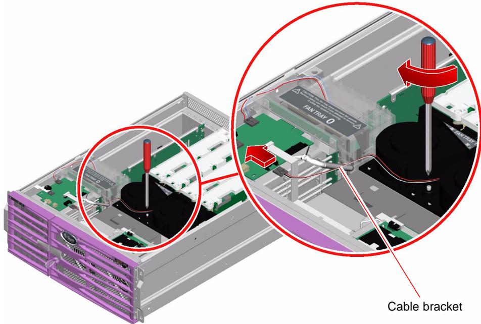
5. **Tuck the cable into the cable bracket on the side of the SCSI backplane.**
