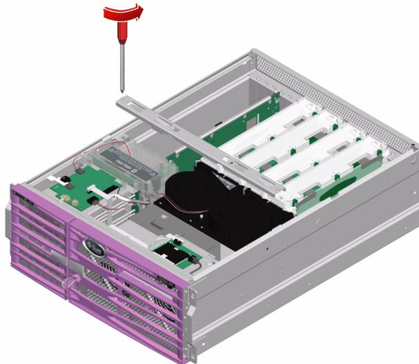
3. Loosen the Phillips No. 2 captive screw securing the CPU fan tray to the chassis.
