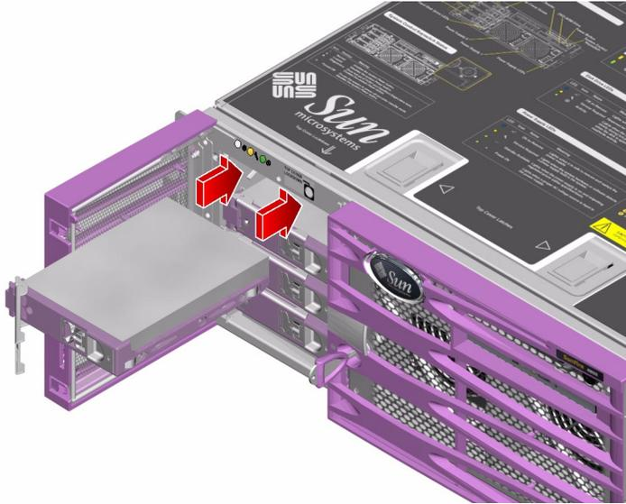
**5. Firmly press the center of the disk drive handle toward the disk drive until the latch closes, securing the disk drive in place.**
