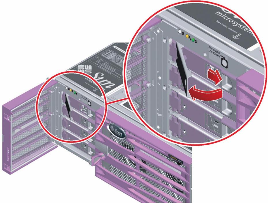
5. Holding the disk drive by the handle, slide the disk drive out of the disk drive bay.
