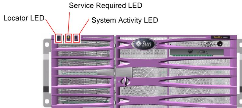
Each system status LED has a corresponding LED on the back panel.
