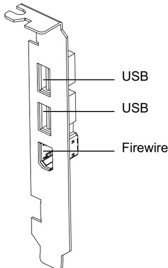
**FIGURE 10-2** SunPCi III USB/Firewire Backplate Connectors
