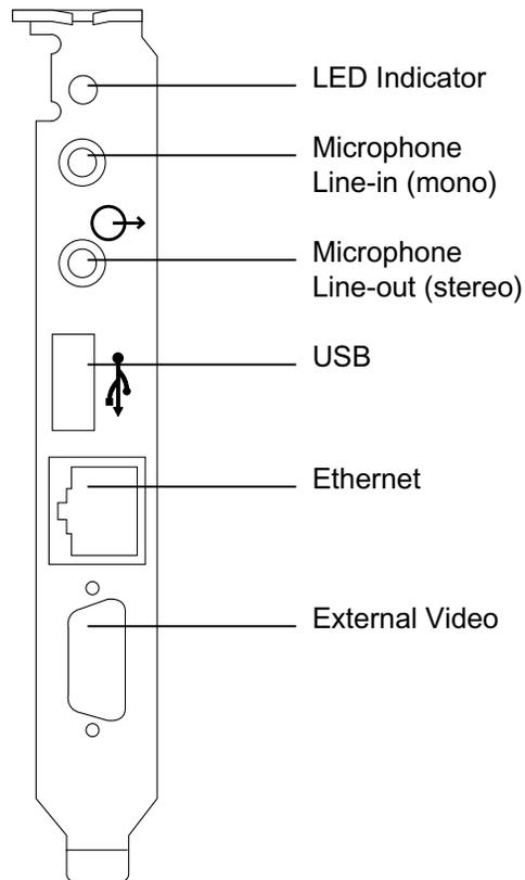
FIGURE 10-1 SunPCi III Main Card Backplate Connectors
