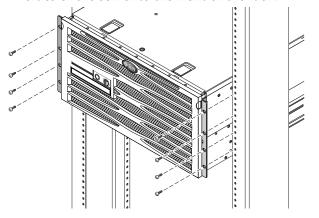
5. Get the two rear mount flanges from the rack kit and, at the rear of the rack, use the two captive screws to secure the two rear mount flanges to the rear mount support brackets that are attached to the server.
