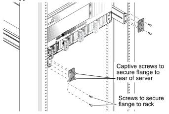
6. Using two screws for each rear mount support bracket, secure the rear mount support brackets to the rear of the rack.
