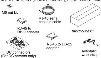
**Note** – The DC connectors are for the DC-powered servers only. Use the separately ordered AC cables with the AC-powered server.
