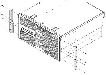
2. Get the two rear mount support brackets from the rack kit and install the rear mount support brackets at the rear of the server.
