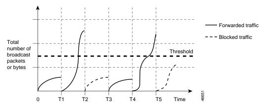
The combination of the storm-control suppression level and the 200-millisecond time interval control the way the storm control algorithm works. A higher threshold allows more packets to pass through. A threshold value of 100 percent means that no limit is placed on the traffic. A value of 0.0 means that all broadcast, multicast, or unicast traffic on that port is blocked.
