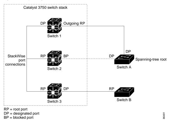
All paths that are not needed to reach the root switch from anywhere in the switched network are placed in the spanning-tree blocking mode.
