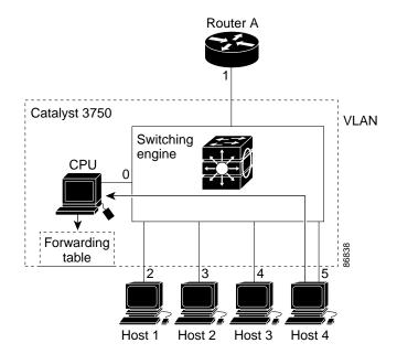
Figure 18-2 Second Host Joining a Multicast Group
