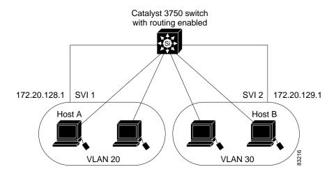
Figure 11-2 Connecting VLANs with the Catalyst 3750 Switch
