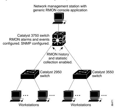
Figure 23-1 Remote Monitoring Example
