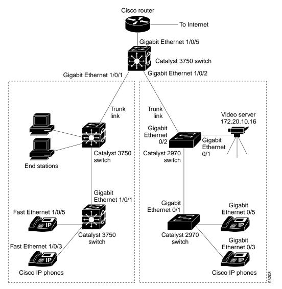
The intelligent wiring closets in Figure 27-10 are composed of Catalyst 2970 and Catalyst 3750 switches. The object of this example is to prioritize the VoIP traffic over all other traffic. To do so, enable auto-QoS on the switches at the edge of the QoS domains in the wiring closets.
