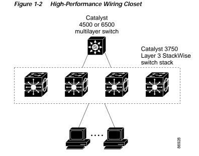
Redundant Gigabit backbone—Using HSRP, you can create backup paths between two
