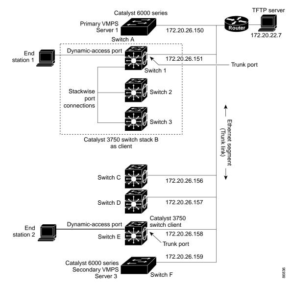
Figure 12-5 Dynamic Port VLAN Membership Configuration
