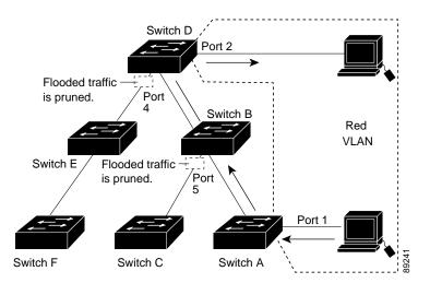
Enabling VTP pruning on a VTP server enables pruning for the entire management domain. Making VLANs pruning-eligible or pruning-ineligible affects pruning eligibility for those VLANs on that trunk only (not on all switches in the VTP domain).
