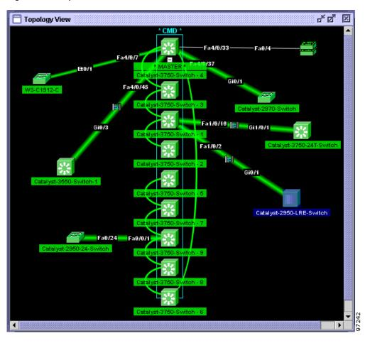
Figure 3-9 Expanded Switch Stack View
