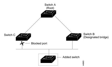
Figure 17-8 Adding a Switch in a Shared-Medium Topology
