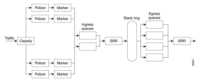
Because the total ingress bandwidth of all ports can exceed the bandwidth of the stack ring, ingress queues are located after the packet is classified, policed, and marked and before packets are forwarded into the switch fabric. Because multiple ingress ports can simultaneously send packets to an egress port and cause congestion, egress queues are located after the stack ring.
