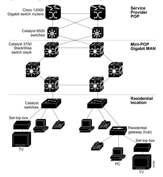
Figure 1-8 Catalyst 3750 Switches in a MAN Configuration
