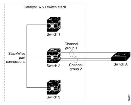
Figure 28-2 Single-Switch EtherChannel
