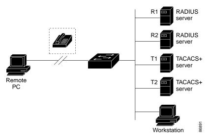
Figure 9-2 Transitioning from RADIUS to TACACS+ Services
