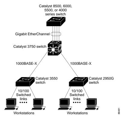
The EtherChannel provides full-duplex bandwidth up to 800 Mbps (Fast EtherChannel) or 8 Gbps (Gigabit EtherChannel) between your switch and another switch or host.
