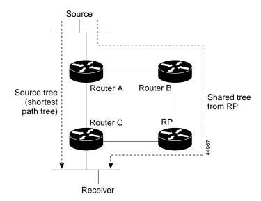
Figure 31-4 Shared Tree and Source Tree (Shortest-Path Tree)
