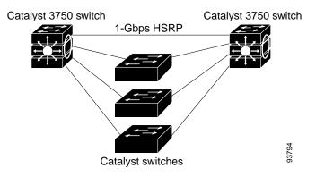
Server aggregation (Figure 1-4) and Linux server cluster (Figure 1-5)—You can use the switches and switch stacks to interconnect groups of servers, centralizing physical security and administration of your network. For high-speed IP forwarding at the distribution layer, connect the switches in the access layer to multilayer switches with routing capability. The Gigabit interconnections minimize latency in the data flow.
