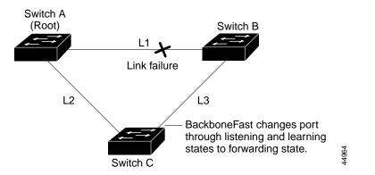
If a new switch is introduced into a shared-medium topology as shown in Figure 17-8, BackboneFast is not activated because the inferior BPDUs did not come from the recognized designated switch (Switch B). The new switch begins sending inferior BPDUs that indicate it is the root switch. However, the other switches ignore these inferior BPDUs, and the new switch learns that Switch B is the designated switch to Switch A, the root switch.
