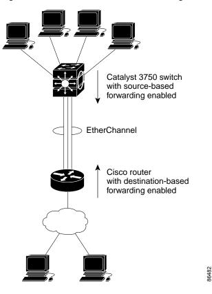
Figure 28-5 Load Distribution and Forwarding Methods
