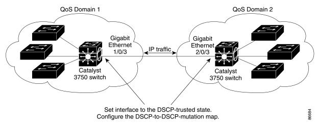
Beginning in privileged EXEC mode, follow these steps to configure the DSCP-trusted state on a port and modify the DSCP-to-DSCP-mutation map. To ensure a consistent mapping strategy across both QoS domains, you must perform this procedure on the ports in both domains:
