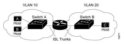
When Host A in VLAN 10 needs to communicate with Host B in VLAN 10, it sends a packet addressed to that host. Switch A forwards the packet directly to Host B, without sending it to the router.
