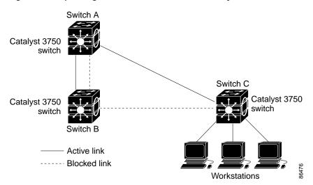
Figure 15-4 Spanning Tree and Redundant Connectivity
