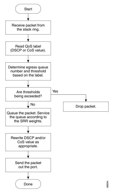
Each port supports four egress queues. These queues are assigned to a queue-set. All traffic exiting the switch flows through one of these four queues and is subjected to a threshold based on the QoS label assigned to the packet.
