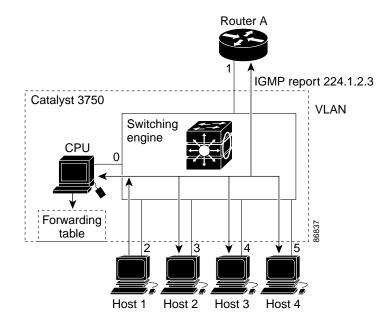
Figure 18-1 Initial IGMP Join Message
