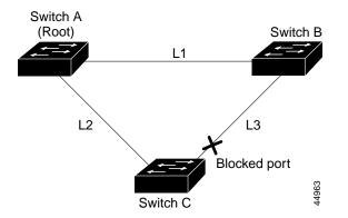
Figure 17-6 BackboneFast Example Before Indirect Link Failure
