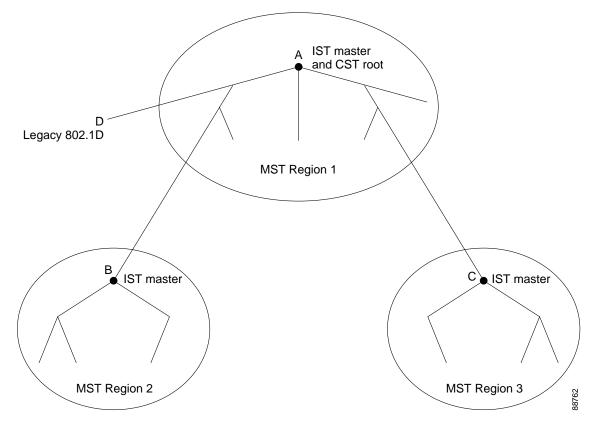
Figure 16-1 does not show additional MST instances for each region. Note that the topology of MST instances can be different from that of the IST for the same region.
