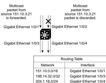
PIM uses both source trees and RP-rooted shared trees to forward datagrams (described in the "PIM DM" section on page 31-4 and the "PIM SM" section on page 31-4). The RPF check is performed differently for each:
