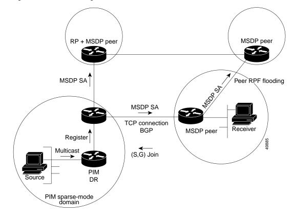
Figure 32-1 MSDP Running Between RP Peers
