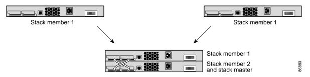
Figure 5-1 Creating a Switch Stack from Two Standalone Switches
