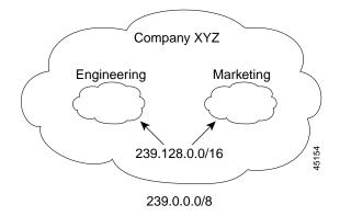
You can define an administratively-scoped boundary on a routed interface for multicast group addresses. A standard access list defines the range of addresses affected. When a boundary is defined, no multicast data packets are allowed to flow across the boundary from either direction. The boundary allows the same multicast group address to be reused in different administrative domains.
