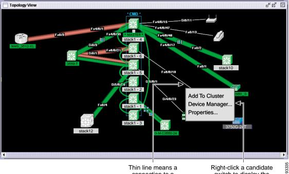
Thin line means a connection to a candidate switch.
