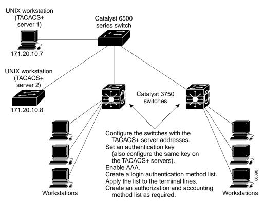
Figure 9-1 Typical TACACS+ Network Configuration
