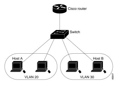
By using the switch with routing enabled, when you configure VLAN 20 and VLAN 30 each with an SVI to which an IP address is assigned, packets can be sent from Host A to Host B directly through the switch with no need for an external router (Figure 11-2).
