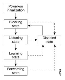
Figure 15-2 Spanning-Tree Interface States
