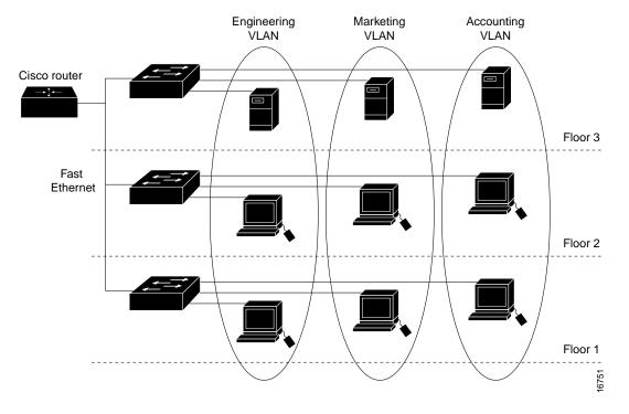
Figure 12-1 shows an example of VLANs segmented into logically defined networks.
