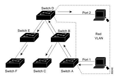
Figure 13-1 Flooding Traffic without VTP Pruning
