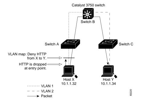
Figure 26-4 Wiring Closet Configuration
