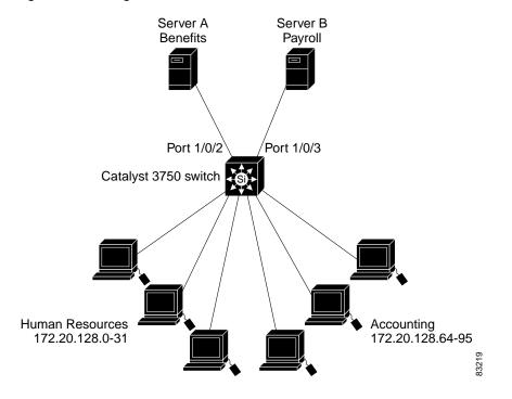
Figure 26-3 Using Router ACLs to Control Traffic
