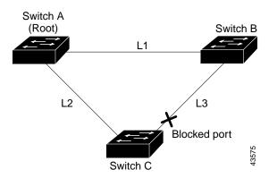
Figure 17-3 UplinkFast Example Before Direct Link Failure
