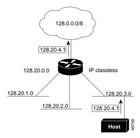
In Figure 29-3, the router in network 128.20.0.0 is connected to subnets 128.20.1.0, 128.20.2.0, and 128.20.3.0. If the host sends a packet to 120.20.4.1, because there is no network default route, the router discards the packet.
