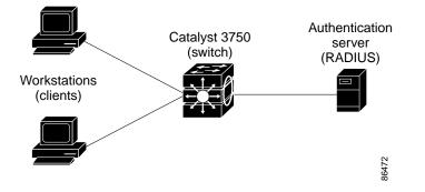
• *Client*—the device (workstation) that requests access to the LAN and switch services and responds to requests from the switch. The workstation must be running 802.1X-compliant client software such as that offered in the Microsoft Windows XP operating system. (The client is the *supplicant* in the IEEE 802.1X specification.)
