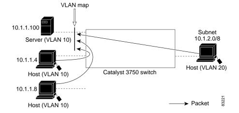
This example shows how to deny access to a server on another VLAN by creating the VLAN map SERVER 1 that denies access to hosts in subnet 10.1.2.0/8, host 10.1.1.4, and host 10.1.1.8 and permits other IP traffic. The final step is to apply the map SERVER1 to VLAN 10.
