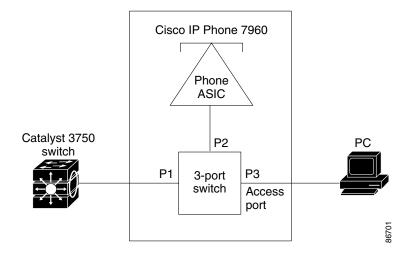
Figure 14-1 Cisco 7960 IP Phone Connected to a Switch
