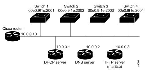
Figure 4-3 DHCP-Based Autoconfiguration Network Example
