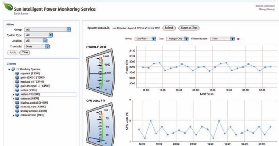
Figure 3-5. Understanding the relationship between power and load utilization helps support workload adjustments
