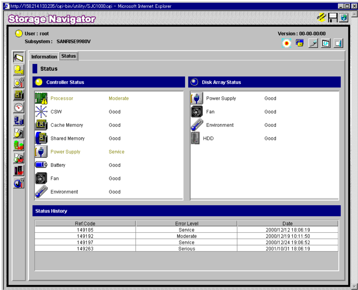
Figure 3.6 Remote Console Main Panel, Status Tab
