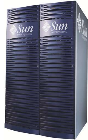
6920 16 6120 Arrays Data Services Platform 1 Service Processor 64 TB 32 GB Cache
