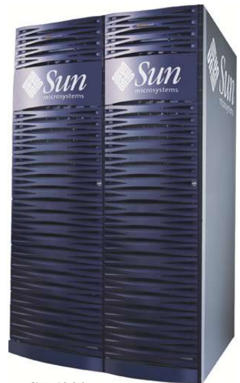
SE6320 22 6020 Trays 1 Service Processor 45 TB 22 GB Cache
