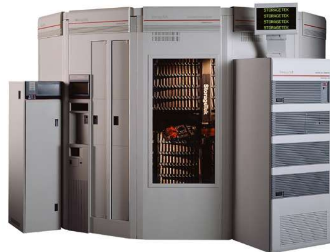
L6000 Tape Library 80 9840, or 80 9940 Drives 6000 Cartridges Can Link 26 L6000's together
