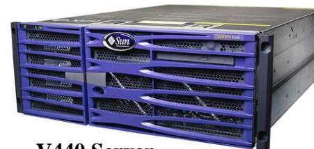
V440 Server 4 USIIIi CPU's - 1.28 GHz 16 GB memory 4 internal 36 GB Disks
