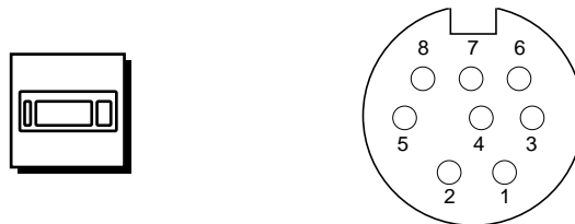
Figure B-1 Keyboard/Mouse Connector Pin Configuration
