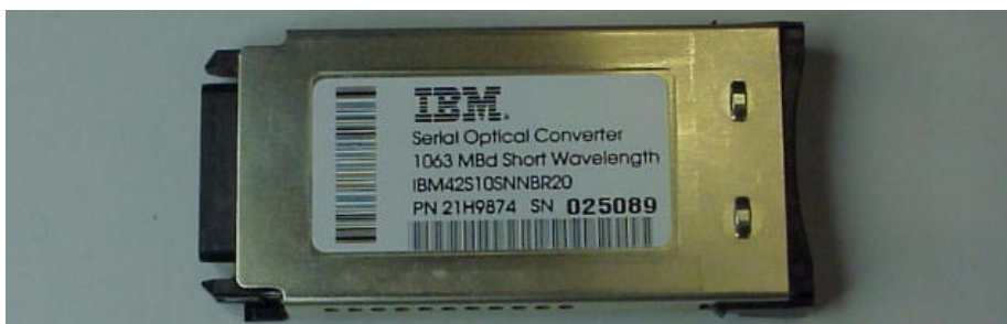
Figure 1-2 Short-Wavelength Laser (SWL) fiber-optic GBIC module
