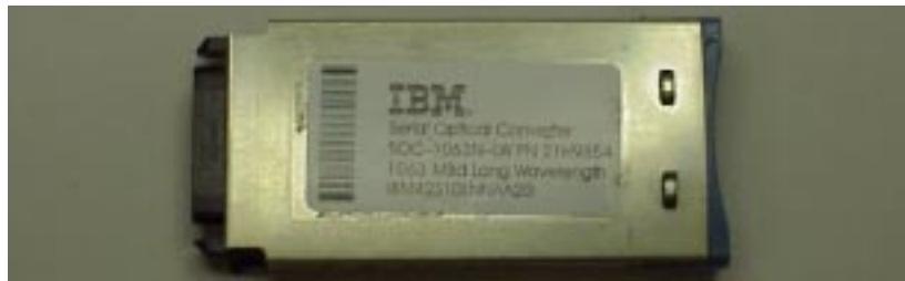
Figure 1-3 Long-Wavelength Laser (LWL) fiber-optic GBIC module
