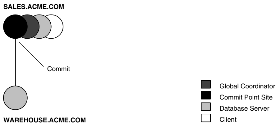
Figure 32–8 Determining the Commit Point Site
