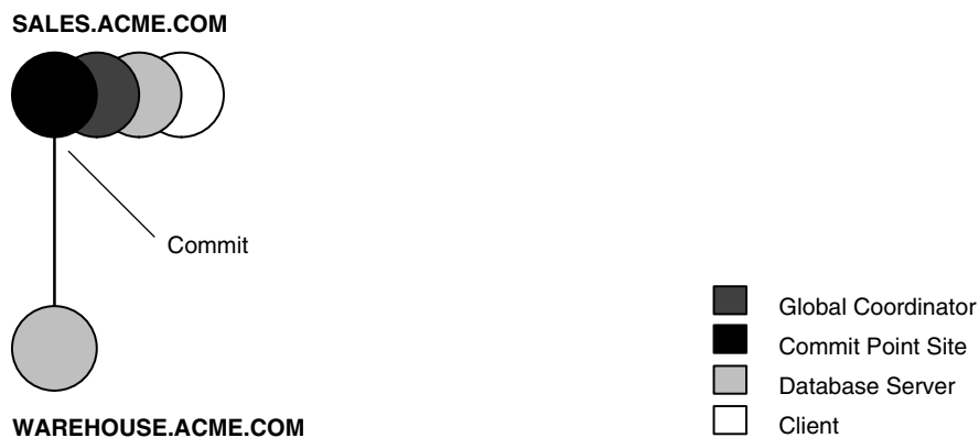
Figure 32–8 Determining the Commit Point Site
