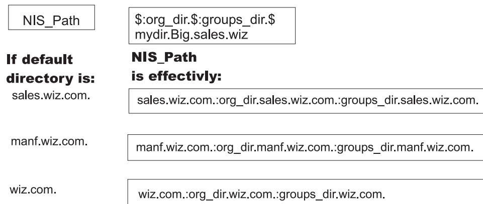
Figure 18. Expanding Directory Pathnames Using NIS_PATH. This illustration shows how search names are expanded by appending each path in the NIS_PATH names. For example, if NIS_PATH is $.org_dir.$:groups_dir.$mydir.Big.sales.wiz , then a default directory of sales.wiz.com. has an effective NIS_PATH of sales.wiz.com.:org_dir.sales.wiz.com.:groups_dir.sales.wiz.com.
