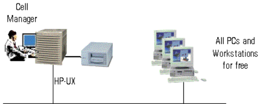
Figure A-3 Cell Manager - Single Drive for HP-UX, Including up to 60 Slot Single Drive Autochangers
