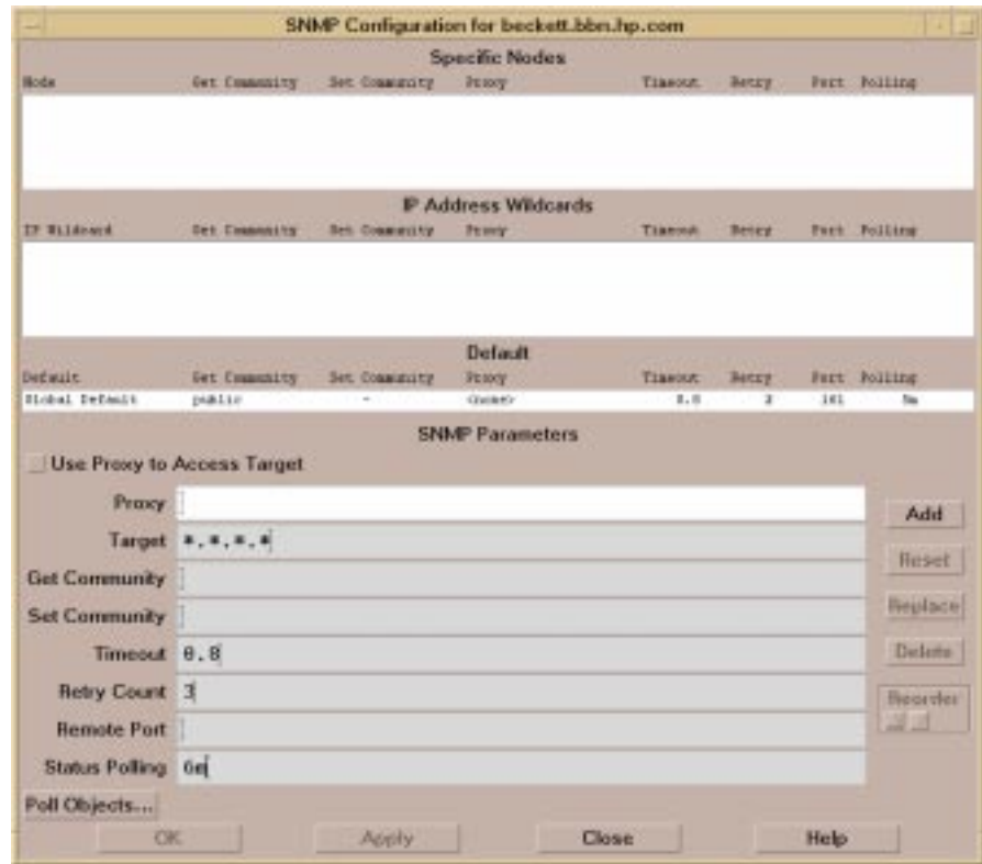
Figure 7-4 SNMP Configuration Using xnmsnmpconf
