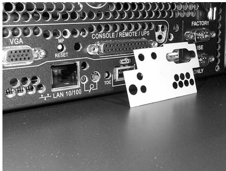
Figure 1-32 Rear Chassis with Port Label Removed
