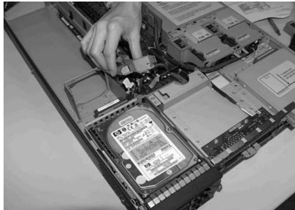
Figure 5-11 Lifting the Fan Power Bridge
