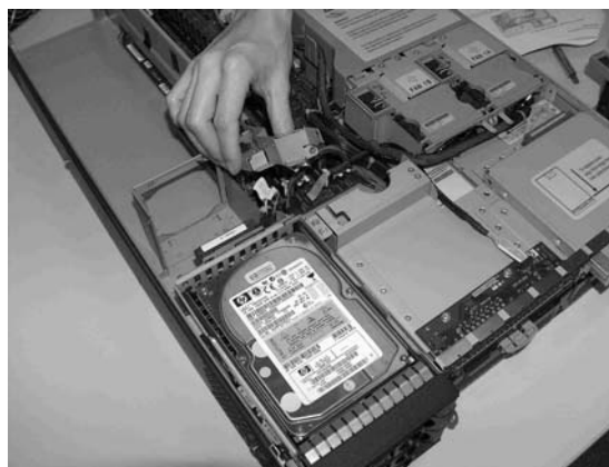
Figure 4-9 Lifting the Fan Power Bridge
