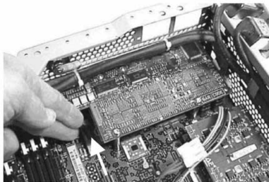
Figure 4-11 Disconnecting the iLO Manageability Card Connector
