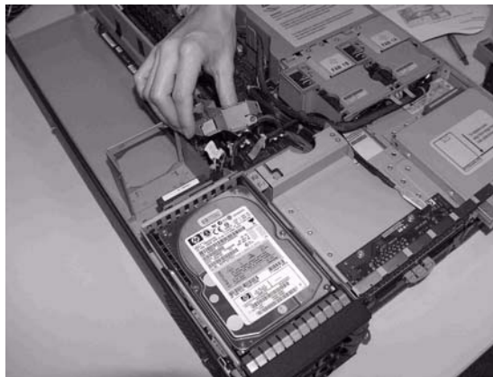
Figure 7-9 Lifting the Fan Power Bridge
