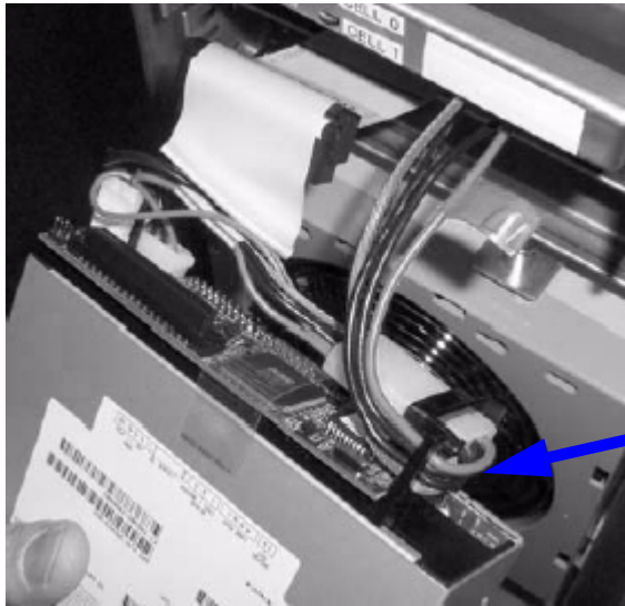
Figure 6-22 Power Cable Connection and Routing
