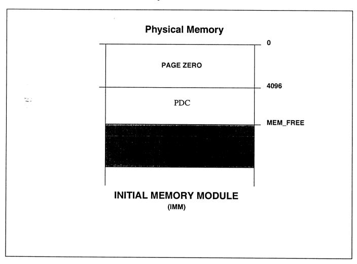
At this point no physical memory has existed for the PDC. The PDC has utilized the area within the EEPROM RAM. The PDC will now allow the CPU to configure and initialize physical memory.
