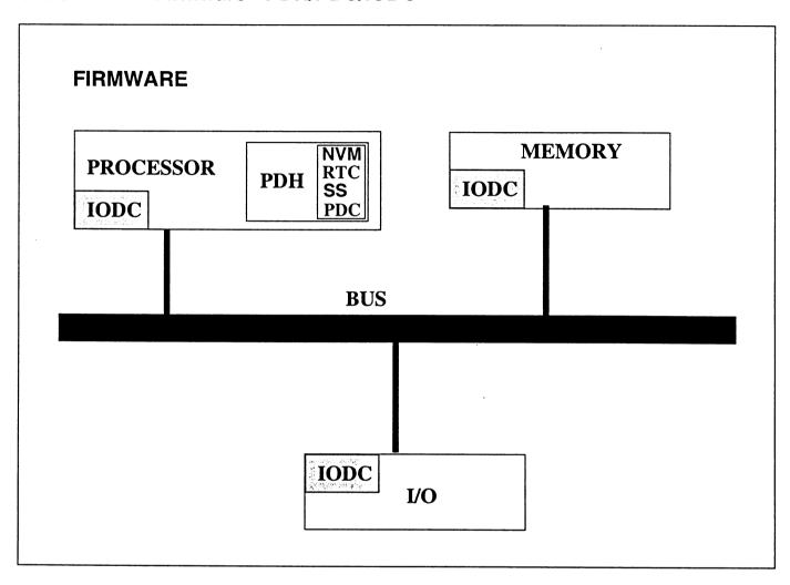
A given system will have several hardware modules, such as processor(s), memory and I/O cards. A module may have different firmware components.
