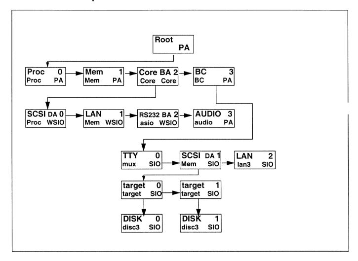
The slide shows an example of the finished product. The I/O tree consists of central data structure of the I/O system based on individual nodes. The nodes provide the hardware path and important information to allow the GIO to manage their configuration.
