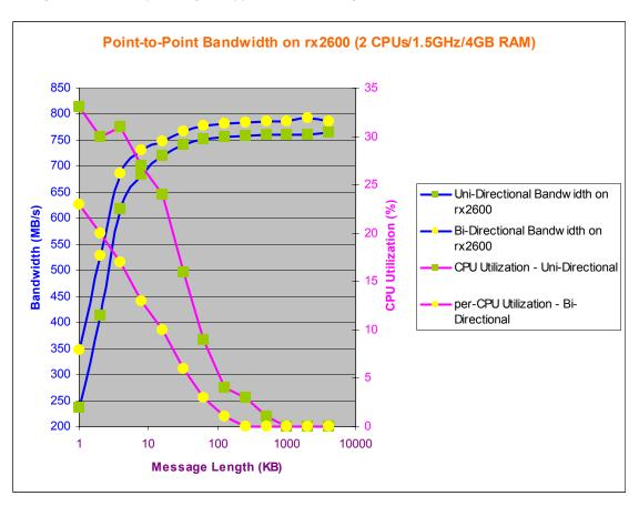
Under bi-directional traffic loads, an acid test for any system performance, HP-UX Fabric Clustering System interconnect solution offers excellent performance results. The bi-directional bandwidth on a rx2600 crosses 731MB/s at a short message length of 8KB with a service demand of only 13% per-CPU utilization. The bi-directional bandwidth is almost equally split across each individual stream for all message sizes.
