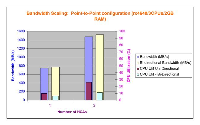
The HP-UX Fabric Clustering System interconnect solution scales without adversely affecting the service demand requirements on the server. Because of lack of dual rope slots on rx4640, HCA scaling was tested only up to 2 HCAs.
