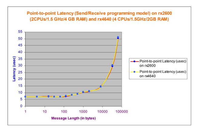
The latency values remain virtually unaffected when the results are obtained from two independent pairs of HCAs plugged into rx4640 servers.
