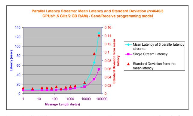
As the number of parallel latency streams, running on the same HCA on a server, start exceeding the number of available processors on the server, process scheduling issues will have an adverse impact on the mean latency and standard deviation values. Process scheduling issues also impact parallel latency streams running on different HCAs, when the number of such streams start exceeding the number of processors on the server.
