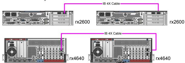
For the HCA scalability tests, 2 HCAs on rx4640 are connected in point-to-point configuration to two HCAs on another rx4640.
