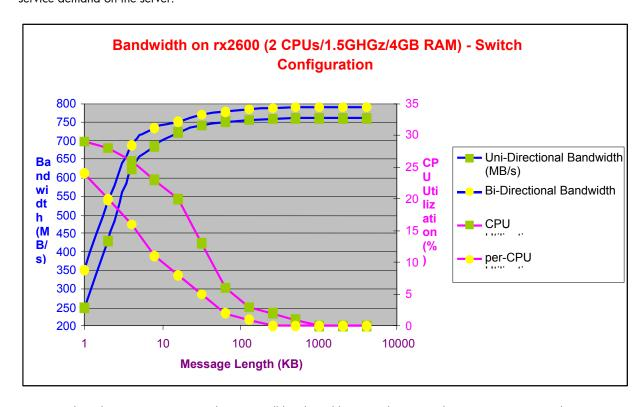
In a typical application environment, the HCA will be shared by more than a single connection. HP-UX cluster interconnect solution scales across multiple connections providing almost an equal share of the available bandwidth for all the parallel connections. On a rx2600 (2 CPUs/1.5Gz/4GB RAM) in a switch configuration, for 32 parallel bandwidth streams, the bandwidth offers a mean bandwidth of 23.67MB/s with a standard deviation of 0.123MB/s, resulting a cumulative bandwidth of 757MB/s.
