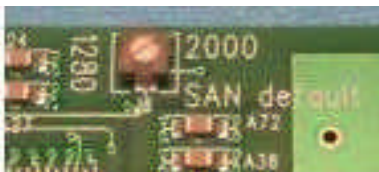
PCI Short card (switch positioned for SAN-2000 rate)
