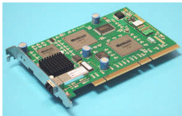
PCI short card (PCI64B, fiber connector)
