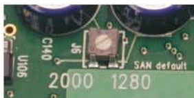
PCI Mezzanine card (switch positioned for SAN-2000 rate)
